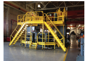
Main Tack Weld Fixtures. No weight or size restrictions. Fixture above holds part weighing 50,000 lbs.
